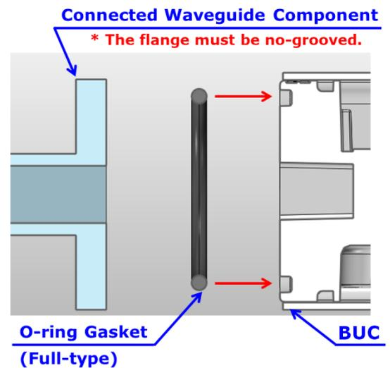
Step 2: Secure the OMT or the filter to the BUC by tightening the enclosed Phillips head screws (M4 x 10 mm) with  $1.52 \pm 0.152$  N·m torque as shown in the figure right, when the thickness of the flange of the OMT or filter is assumed to be 3 to 5 mm. The enclosed washers as accessory must be inserted to bolts before tightening bolts.
